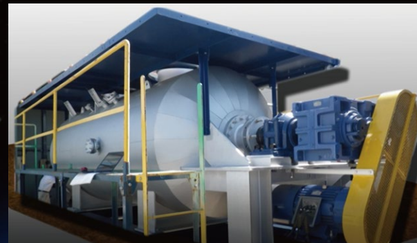
The ALIN 10 model can process 7m 3 of waste per cycle.
